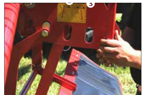
All centre swath rakes have variable working width. On R+ 760 you can remove the canvas and use the hole to get an even smaller working width. This could be relevant when working in alfalfa.
