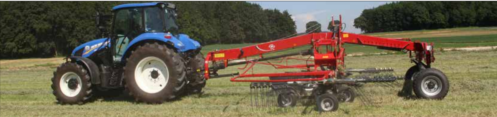
R+760 - trailed centre swath rake (working width 6.5-7.6 m).
