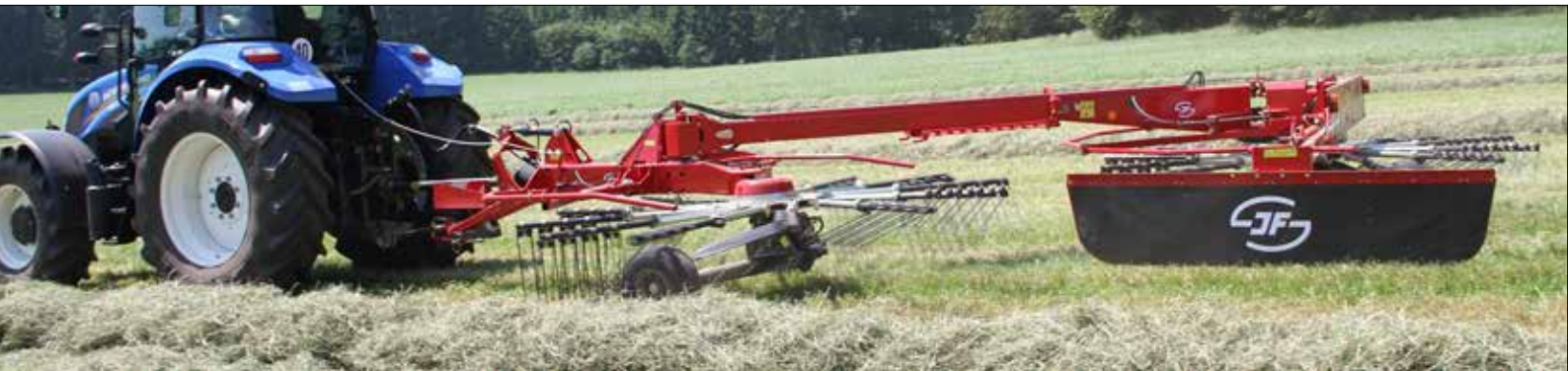
R+ 1410 S - a side delivery rake with Multi Link frame
