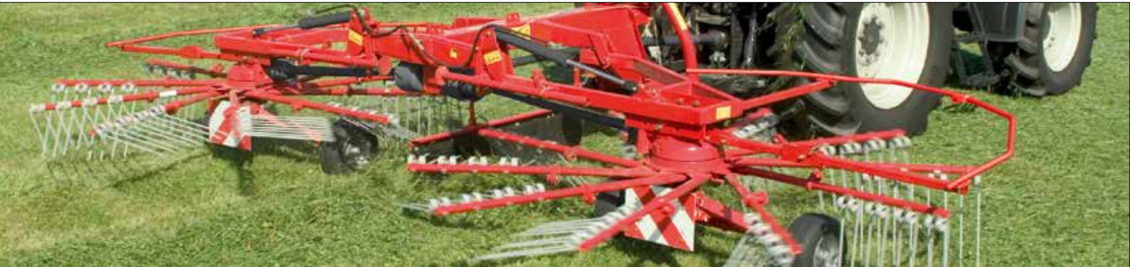
R655 DS - 3-point mounted centre swath rake.
