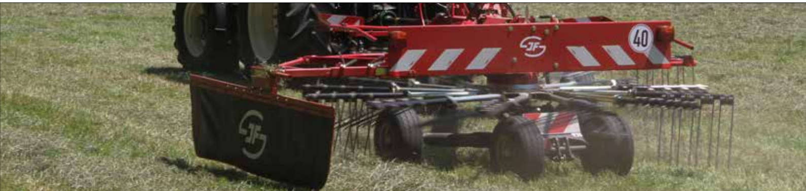
R+ 1410 SB - a side delivery rake with Multi Link frame
