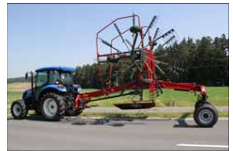
R+ 760 in transport position. The transport height is under 4 m.
