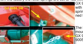
GX 9005 SM (i.e. with conditioner) the springs must be tightened to 400 mm.
